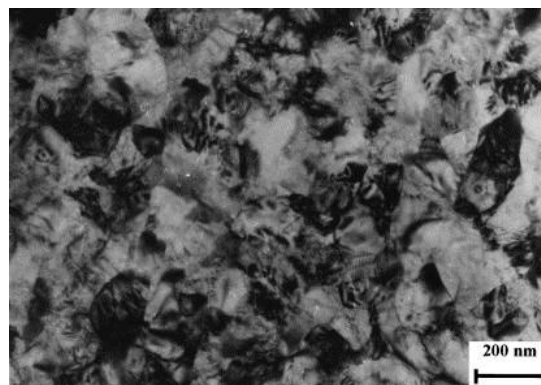
Figure 2.8: TEM micrograph of titanium subjected to severe torsion straining [12].
